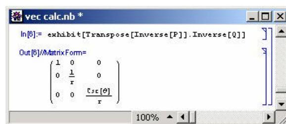
Figure 4. Computation of coefficient matrix for spherical polar form of **grad**.
