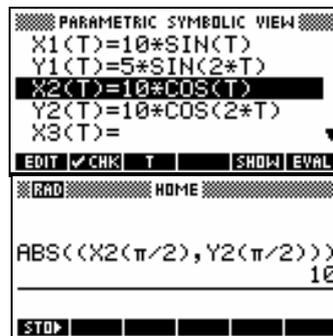
Figure 5. Calculating speed by naming the location of the velocity components.
