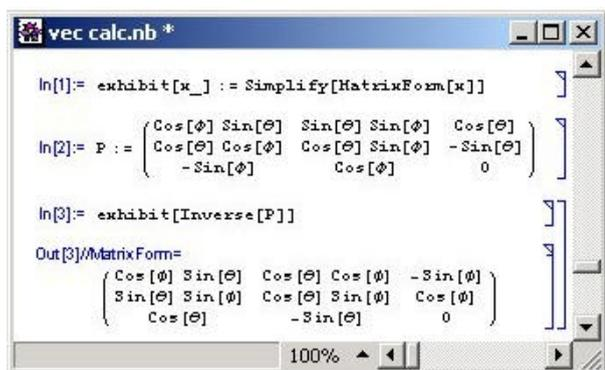
Figure 2. Inversion of spherical polar coordinate matrix
