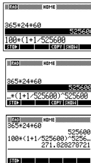
Figure 2. Transporting values by using the COPY capability.
