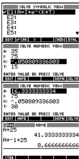
Figure 4. Calculation using the value in memory 'A'.
