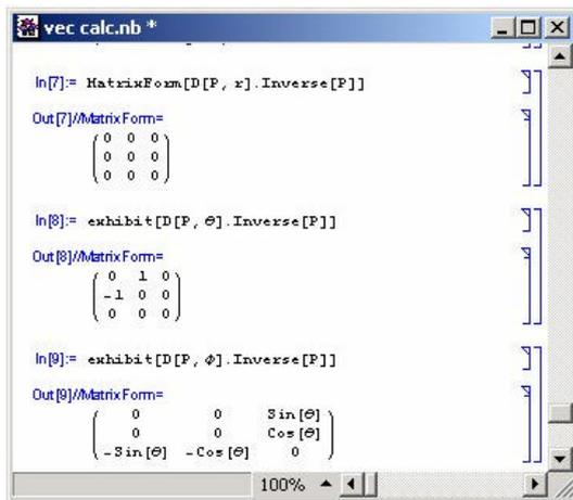
Figure 5. Computations of rate of change of polar unit vectors in terms of the polar coordinates
