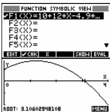
Figure 11. Solving  $f(t) = 10 + 12t - 4.9t^2$  using the graph and ROOT command.
