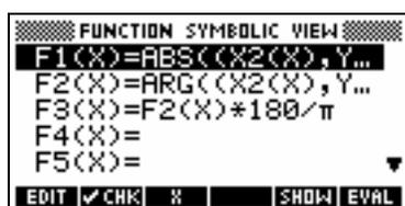
Figure 7. Speed F1(X), argument in radians F2(X) and argument in degrees F3(X). The calculator was set in radians. F1(X)=ABS((X2(X), Y2(X))) and F2(X)=ARG((X2(X), Y2(X)))
