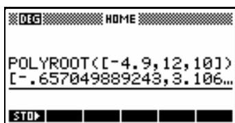
Figure 10. Solving  $f(t) = 10 + 12t - 4.9t^2$  using POLYROOT
